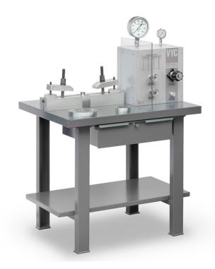
The test is designed to test the safety valves with flanges up to a nominal diameter of DN 125/5".
