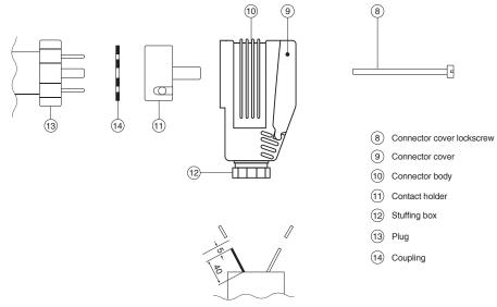
· Make sure the coupling (14) is correctly positioned.
