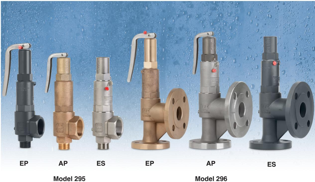
The valve works as an automatic pressure releasing regulator activated by the static pressure existing at the entrance to the valve and is characterized by its ability to open, at the first proportional to the pressure increase, and after instantly and totally.
