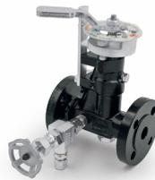
The continuous blowdown valve discharges an adjustable quantity of water from the steam boiler, thus removing organic materials, dissolved mineral salts, suspended solids, etc. With the blowdown process, we prevent damage caused by corrosion and perforation and reduce incrustations, sediments and foam formation inside the boiler.
