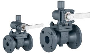
Valve designed for feed water treatment. The valve allows the elimination of excess salts in the water inside the boiler, thus reducing bubbles and foams, and consequently avoiding the appearance of sludge and lime scale generated by the salt inside the boiler, as well as purging it of other particles of dirt and impurities. Bleeding valves for steam boilers prevent early deterioration of the boiler.
