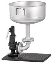
During the expansion process of compressible media such as vapour or gases, one of the main disadvantages is noise pollution. The noise is caused by opening the valve and discharging the expanded fluid at sonic velocity. Silencers are the great alternative to attenuate the noise at the valve discharge and leave it at permissible levels. Noise reductions of more than 50 dB are achieved without additional sound absorption materials.
