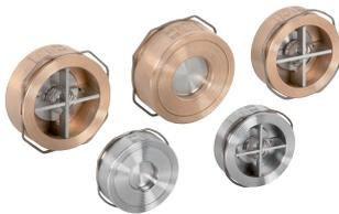
Disc check valve with centering ring for placing between flanges in accordance with DIN, UNE, ANSI, BS, etc. DN -15 to 100. Face-to-face dimensions in accordance with EN-558, basic series 49.
