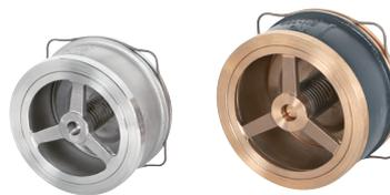
Disc check valve with centering ring for placing between flanges in accordance with DIN, UNE, ANSI, BS, etc. DN -125 to 300. Face-to-face dimensions in accordance with EN-558, basic series 49 and 51.
